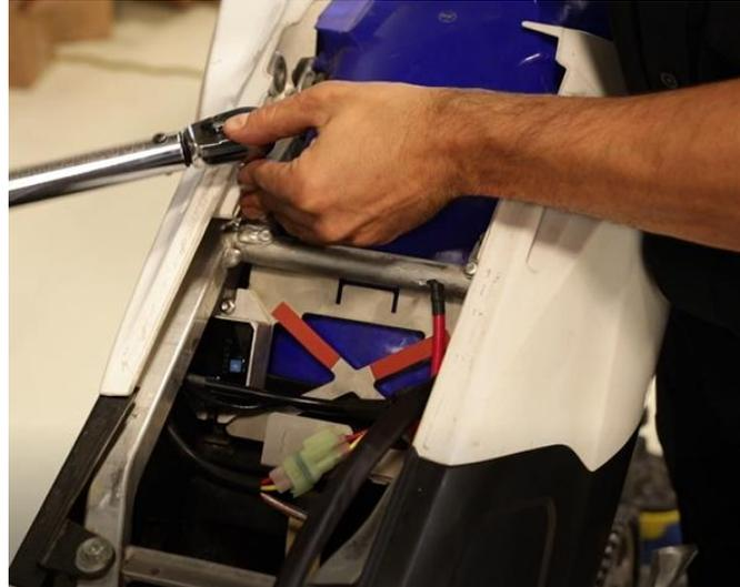
Install the battery box inside the airbox and bolt it to the subframe holes available. Use the 2 supplied M8 socket bolt and spacer and torque to 110 in-lb.
