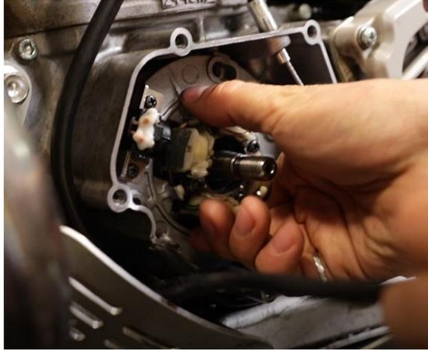
With a philips drive bit, remove the 5 flywheel cover bolts and cover.
