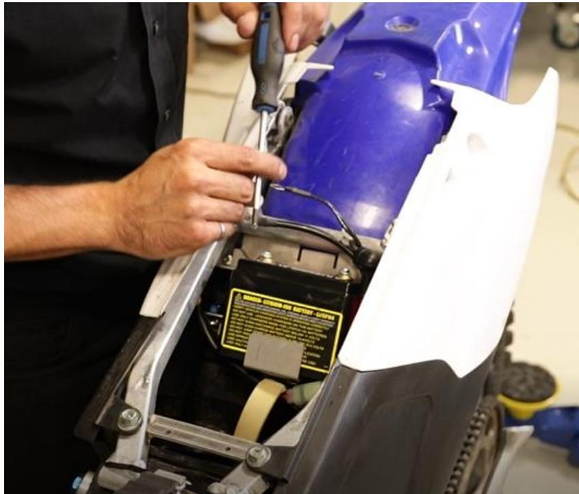
Connect the harness to the battery, always connect the positive (red) first.
