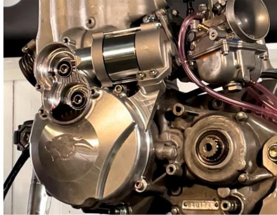
To install the cover, remove the two small gears from behind the gears cap. Leaving the gears will make it hard to put the cover on and align the gear at the same time, you will risk damaging the gears.
