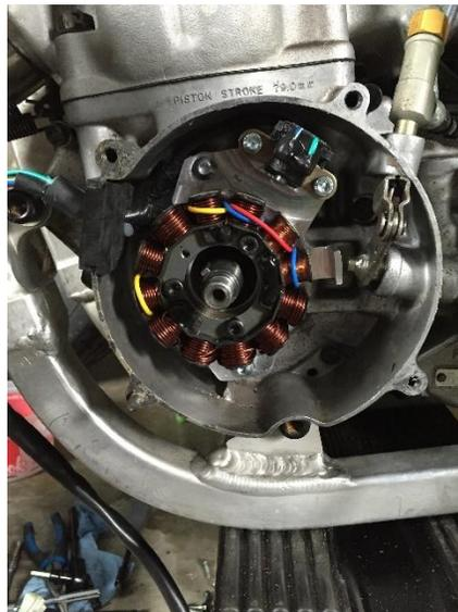
*Figure 2 Stator installation*
