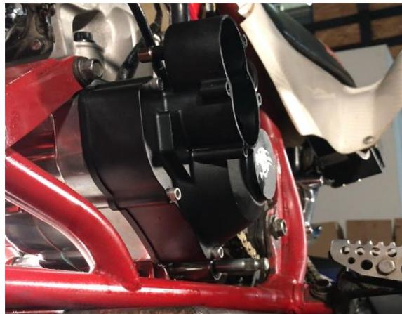
Make sure the main gear is still spinning freely clockwise after the cover is torqued in place.
