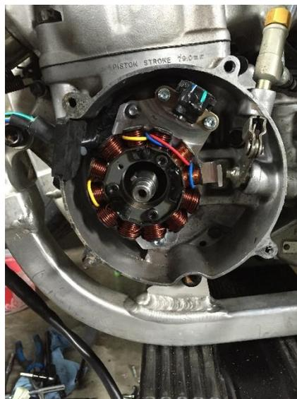
*Figure 2 Stator installation*
