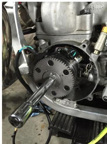
*Figure 3 Flywheel torquing*
