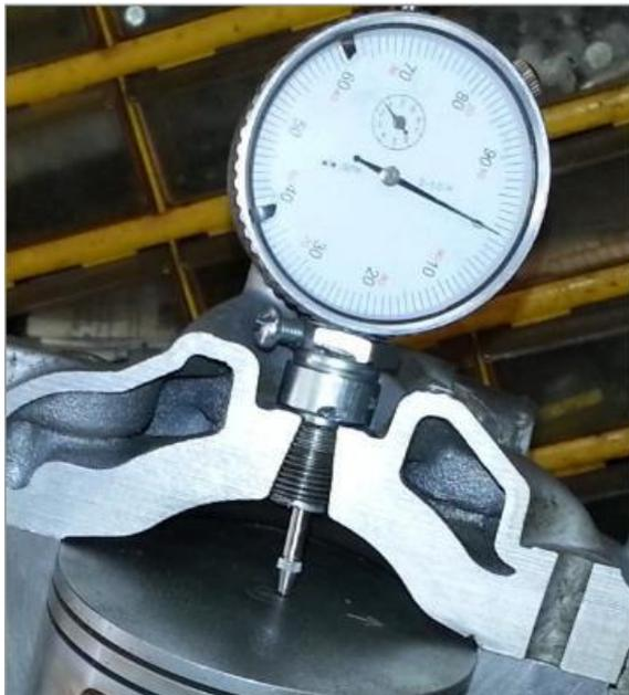
Take the spark plug out to ease turning of the crank and bring the piston into ignition position (put the rotor loosely onto the crank shaft and using it as a turning knob). Please consult your manual of the bike.
