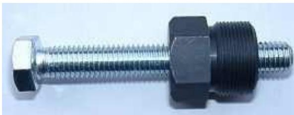
To disengage your new rotor again, you will need a puller M27x1.25 (part-no.: 99 99 799 00 -**Not provided!**-).
