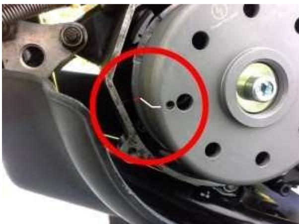
Carefully remove the rotor again from the crank (best using the puller tool for this) and reset it in such a way that the marking on the rotor aligns with the (transferred) marking of the stator. If there is any change in the crank's (ignition) position, you have to start again.
