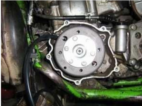
In this position fasten the rotor carefully with the screw provided.
