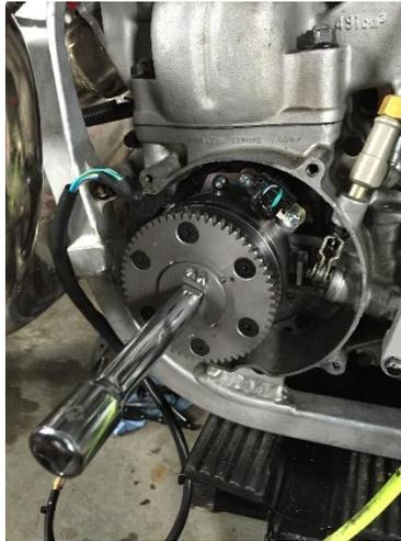
*Figure 1 Flywheel torquing*
