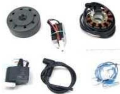
Magnet based generator with integrated fully electronic ignition. Output at 12V/100W DC. Solid state ignition with own power supply from within the system. Replaces old magneto, pickup, regulator and ignition coil.
